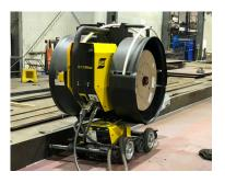
Versotrac enables orienting the welding head for fillet or butt welds and the flexibility to quickly adapt to different beam configurations. The PEK controller communicates more welding & process data, improving traceability.
