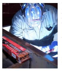
With competitive units, operators had full access to make adjustments to voltage and wire feed speed. As a result, instead of taking the time necessary to climb out of the pit, they would often use sub-optimal settings. Now all the operator only has to focus on travel speed and gun technique, so WPS conformance is more assured.
